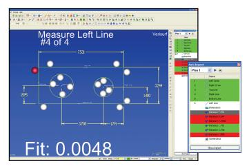
Simply measure the part once. When you create the report, nominal values and tolerances are automatically taken from the CAD model (or input from blueprints). Complete the plan by selecting a format and choosing which properties to report. The next time you want to inspect the same part, just run the plan and print the results.
