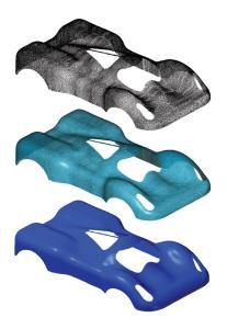
Verisurf *Reverse* offers today's most advanced and powerful CAD/CAM software tools for processing 3D scan data into usable manufacturing models. It brings state-of-the-art technology to the RE process by utilizing direct measurements of a physical part or artifact to produce an accurate, replica 3D CAD model.
