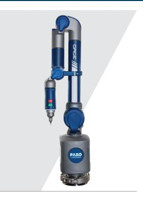
The all-new FARO® Gage is our most affordable 3D Coordinate Measuring Machine (CMM). It is also the most accurate FaroArm ever produced, and allows for confident measurements across a wide range of industrial uses at a value that delivers a significant return on investment (ROI).
